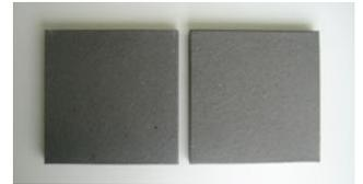
Ceramic tiles made with powder generated during production of recycled aggregate (used in the floor of the building pictured at the left)
