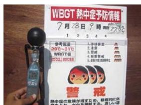
WBGT meters installed at construction sites
