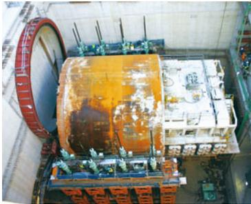
Looking down on the shield machine from ground level. With a diameter of 13.6 meters, it is the largest of its kind in Japan, in terms of mud pressure.
