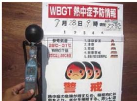
WBGT meters installed at construction sites
