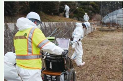
Identifying decontamination status using a buggy-type radiation measurement system equipped with GPS
