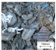
A mixture of concrete rubble wood rubber metals, earth and rock, plastic, tiles, and other materials (ranging between 25-150mm in diameter)
