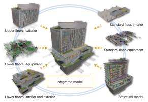
An integrated model (the *oak omotesando* building) combining three-dimensional models of the structure, equipment, exterior, and interior. We made extensive use of this model during the construction process review and other phases of the project.
