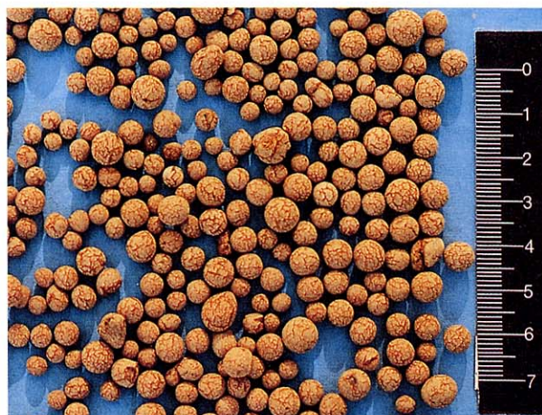
Photo 3 超軽量粗骨材「リアポール」 Ultra-Lightweight Coarse Aggregate "Liapor"
