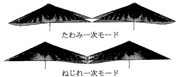
Fig. 2 振動モード First Eigenmodes for Vertical Bending and Torsion
