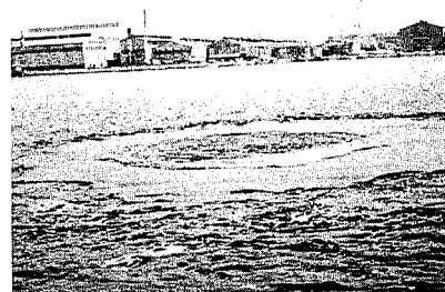
Photo 3 気泡弾による底層水の揚水 Scene of Flowing Up the Lower Water with the Crowd of Air
