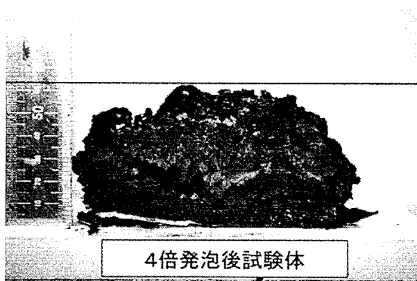
Photo 1 PIBゴム発泡後の様子 Photograph of Expanded PIB Rubber
