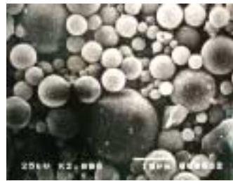
Photo 3 石炭灰 SEM Picture of Coal Fly Ash
