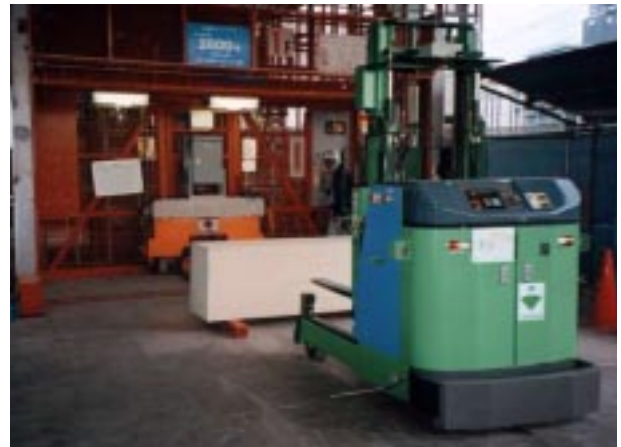
Photo 2 自動移載装置とA G F Automatic Unloader and Automatic Guided Fork-lift
