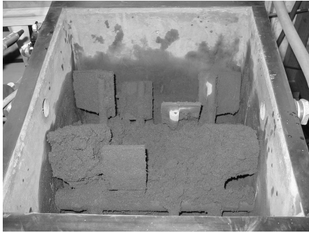
Photo 1 容器内汚染土の様子 (山砂) Sandy Soil in a Container of the Apparatus
