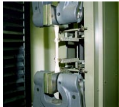
Photo. 5 引張試験の状況 Testing of Tensile Strength
