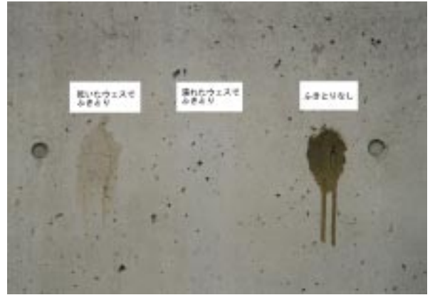
Photo. 3 樹脂を付着させた時の汚れ具合 Dirty Level on the Wall Attached Epoxy Resin
