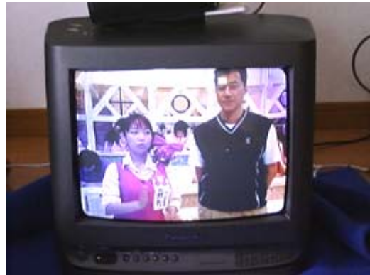
Photo 4 色ずれ障害(TV画像) TV Screen Color Error (Real Television Image)
