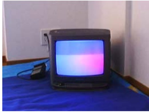
Photo 3 テレビ本体の脱磁後(点A 2) After demagnetizing from Television at Point A2
