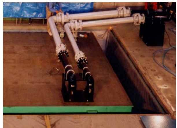
Photo 3 免震配管性能実証試験の一例 Vibration Test of Isolation Equipment
