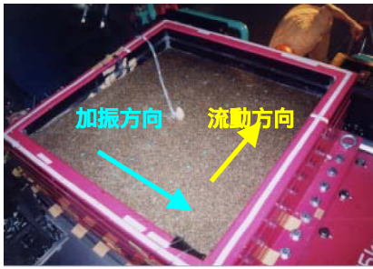
Photo 2 側方流動実験の地盤模型 Model Ground on the Centrifuge Shaking Table
