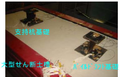
Photo 6 杭併用直接基礎 Piled Raft Foundations
