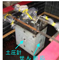
Photo 5 複合基礎 Composite Foundation
