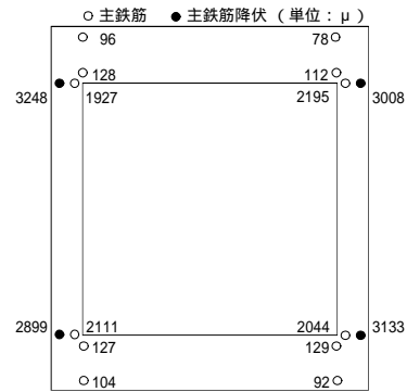
Fig. 15 鉄筋の最大ひずみ (25G入力) Distribution of Max. Strain in Bar (25G Input)
