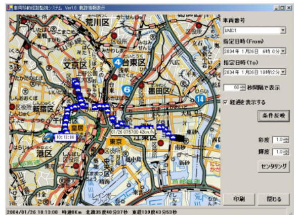
Fig. 13 回収車輛の運行軌跡管理画面 Check for Recovery Tracks Route of Construction Waste via Internet
