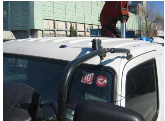
Photo 5 廃棄物回収車輛へのGPSアンテナ取付状況 Global Positioning System on Recovery Track of Construction Waste
