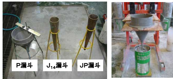
Fig. 5 各種漏斗試験器および圧縮強度供試体作製状況 Funnel Test and Production of Strength Specimens
