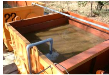
Photo 1 実証試験で用いた鉄粉反応槽 Iron Powder Reaction Tank at Field Test
