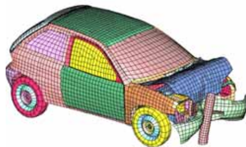
Fig.5 車両停止バリアの性能検討例 Simulation on the Performance of Vehicle Stop Barrier
