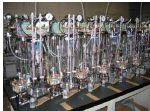
Photo 1 透水試験状況 Appearance of Hydraulic Conductivity Test
