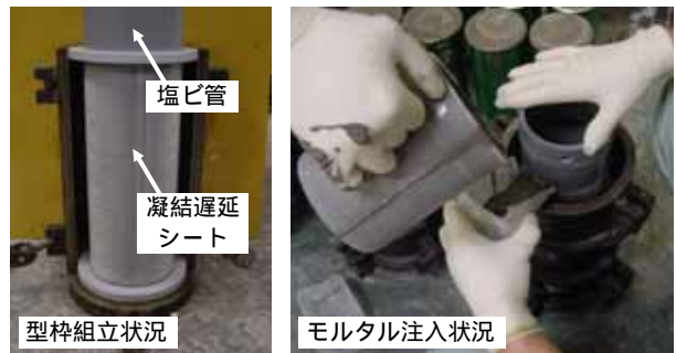
Fig. 4 プレキャスト型枠の作製状況 Production Procedure of Pre-cast Form
