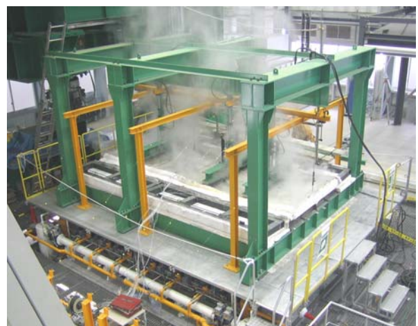
Photo 7 合成スラブの荷重加熱実験の状況 Heating State of Slab Specimen
