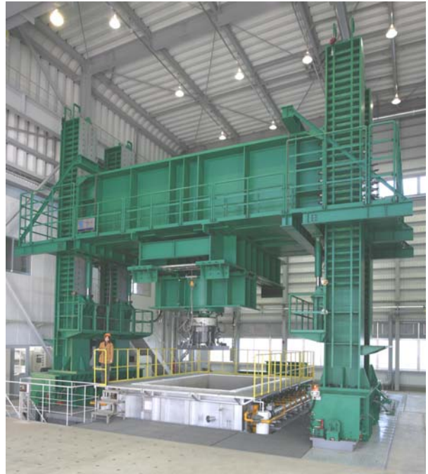
Photo 5 20MN 載荷装置 Loading Apparatus (Loading Capacity: 20MN)
