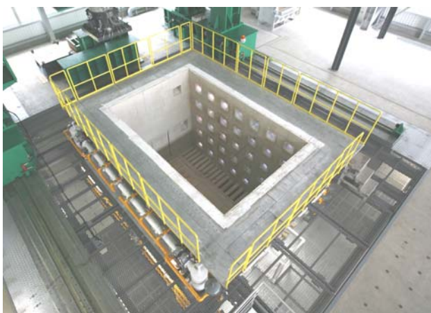
Photo 3 汎用耐火炉 (1F床レベルより俯瞰) Multipurpose Fire Resistance Test Furnace
