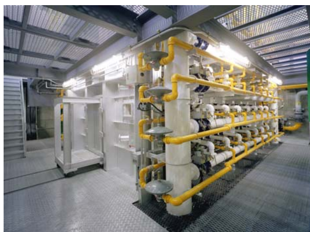
Photo 4 汎用耐火炉 (地下ピット内) Multipurpose Fire Resistance Test Furnace
