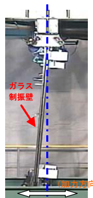
Fig.7 加力状況 Loading Situation (面外加力) (Out-of-Plane Load)
