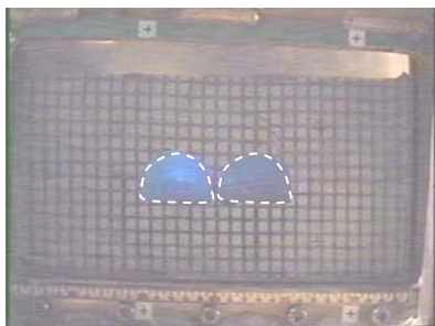
Photo 5 変形結果(43G) (Case2) Ground Deformation at 43G
