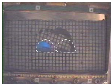
Photo 6 変形結果(44G) (Case2) Ground Deformation at 44G
