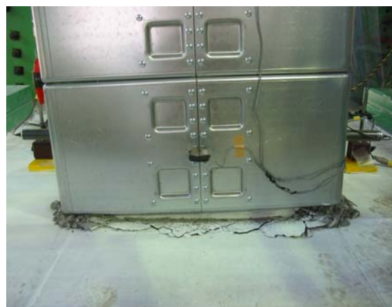
Photo 4 8 y時の塑性ヒンジ部状況 (D試験体) Circumstances of Prastic Hinge at 8 y(Specimen D)
