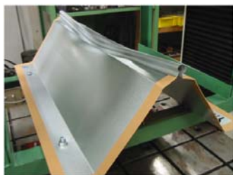
Photo 1 二重折板試験体の引張り試験 Tension Load Testing of Double-Deck Panel
