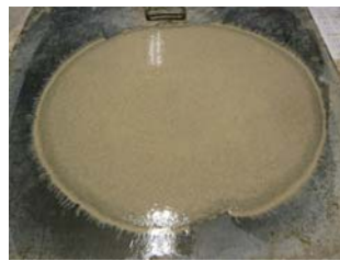
Photo 9 分離状況 Segregation of Materials
