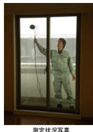
Fig. 8 窓サッシの遮音診断測定例 A Measurement of Sound Insulation of Window Sash
