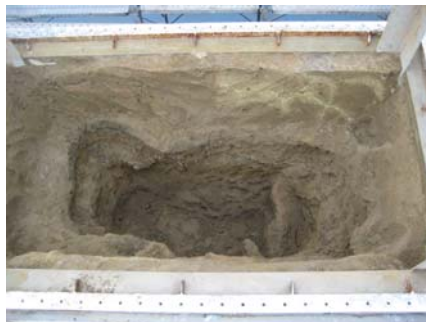
Photo 10 1次注入体の露頭状況 Externals of Infiltration Layer Formed the First Injection
