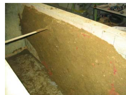
Photo 9 1次+2次注入した注入試験(ケース5) Situation of Injection Test does the First Injection and the Second Injection (Case5)
