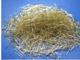
Photo 1 高強度鋼繊維 High-Strength Steel Fiber
