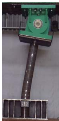
Photo 3 破壊状況 (長柱曲げせん断実験) Failure Mode of Beam Column Tests
