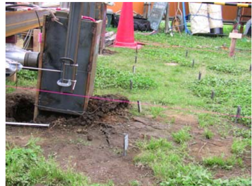
Photo 1 載荷実験状況(杭No.1, 根固めなし) State of the Test (Pile No.1)
