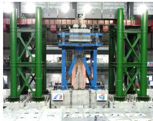
Photo 1 実規模橋梁耐震実験の状況(E-Defense) Set-up using E-Defense shake table(E-Defense)
