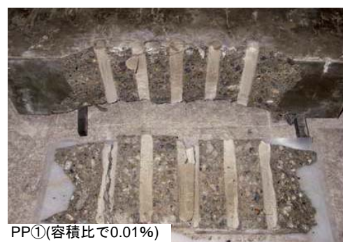
Photo 4 打撃試験後のはく落状況の例 Example of Coming off Situation after Shock Test
