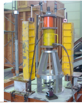
Photo 2 定着強度確認試験状況 Anchorage Strength Confirmation Examination
