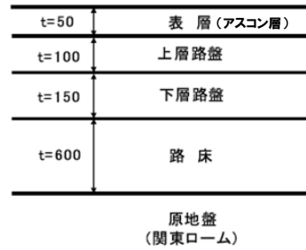
Fig. 8 舗装構成 Pavement composition of field test layer
