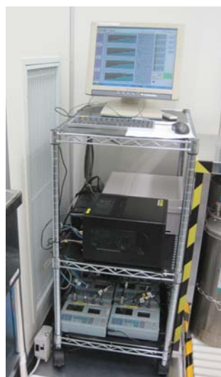
Photo 1 監視装置本体外観 Vibration Monitoring System
