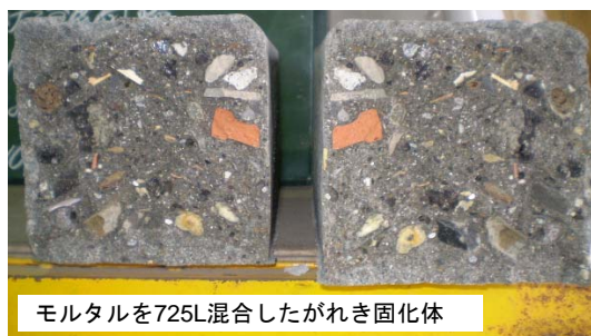
Photo 6 曲げ試験後の破壊面の状況 Situation of Destructive Section after Flexural Strength Test
