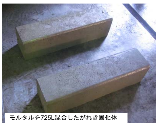
Photo 5 即脱後の表面の状況 Situation of Surface after Immediate Demolding
