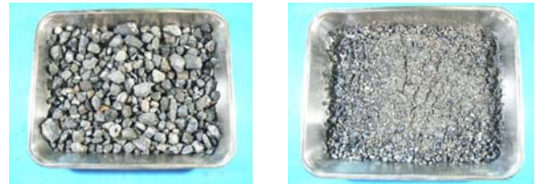
Photo 4 再生骨材(左:粗骨材, 右:細骨材) Recycled Coarse Aggregate and Fine Aggregate
