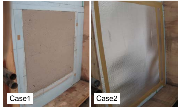
Photo 1 養生シートの貼付け状況 Attachment Situation of Curing Sheet
