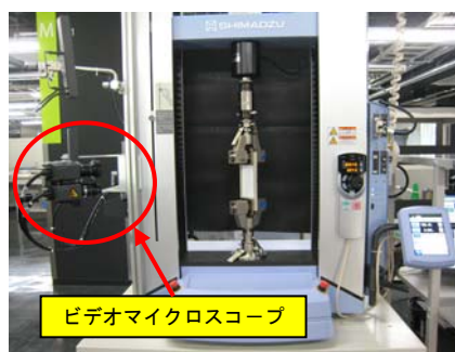
Photo 3 ひび割れ追従性試験の様子 Condition of Crack Bridging Elongation Test
