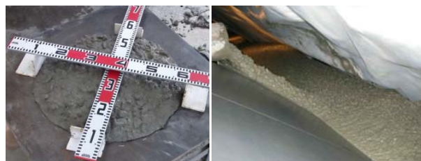
Photo 1 スランブフロー試験状況(左)と流動状況(右) Slump-Flow Test and Flowing Situation of 'Smooth-Crete'
