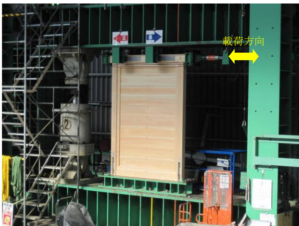
Photo 2 実大加力実験状況 Set up of Full-Scale Specimen and Loading Machine
