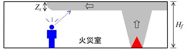
Fig. 7 煙拡散の概念図 Conceptual Diagram of Smoke Diffusion
