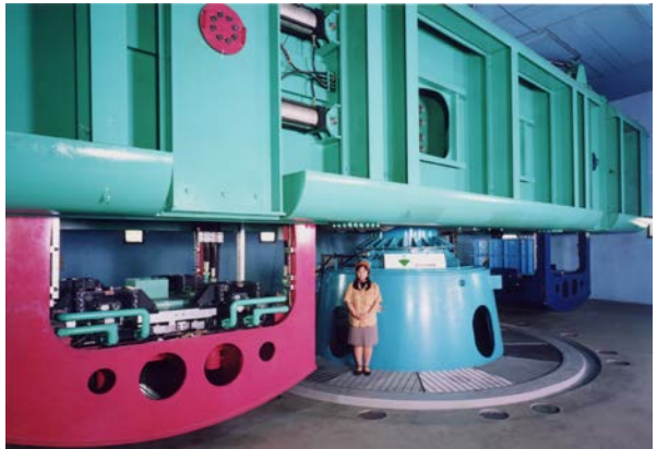
Photo 1 遠心模型実験装置 Obayashi Centrifuge Facility
