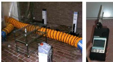
Photo 2 ベークアウトの状況(左)とニオイセンサ(右) The situation of Bake Out (left) and a Odor Sensor (right)
