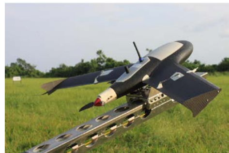
Photo 1 UAV射出時の状況 Picture of Launching UAV
