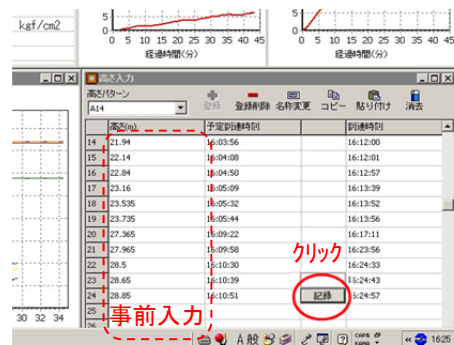
Fig.9 パソコンへの高さの記録方法 Record of the Placing Height to the Personal Computer
